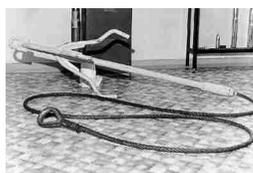
Fig. 2 The trawl wire cutter. (Landhelgisgæslan, Ísland)
